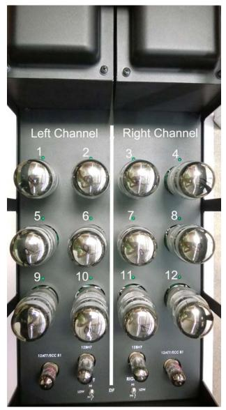
1. Plugging in a new tube: Hold onto the upper portion of the tube towards its tip. Lower the tube onto the socket, making sure that the pins from the tube match the holes in the socket.
